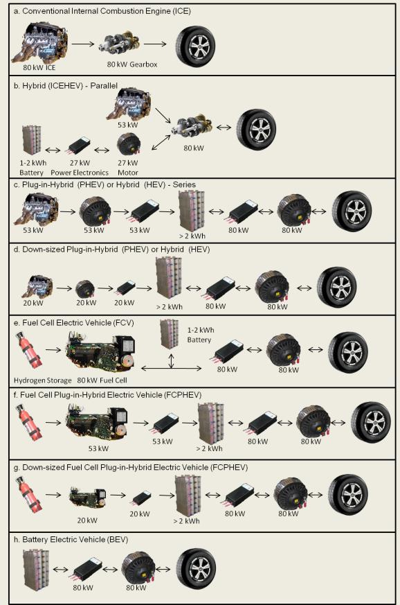
Figure 3. Diagram describing the eight vehicle platforms selected for analysis in the paper; power figures (in kW) are relative to the multipurpose vehicle.
